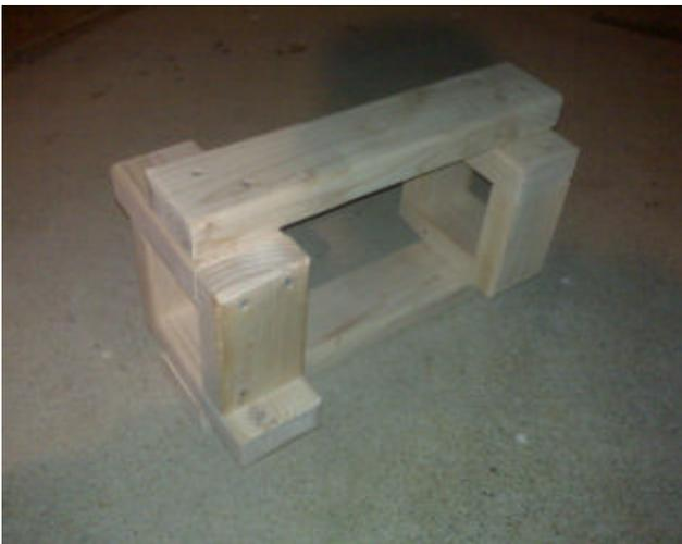
Attach each of the boxes to opposing ends of the two 16-7/8 inch pieces, centering the 16-7/8 inch pieces on the side of each box and lining up the ends of the long pieces with the top of one box and the bottom of the other. Note that the hole in the center of each box is slightly larger than the width of the 2" X 4", so you do not want the seam of the box side to line up evenly with the edge of the 2" X 4"
