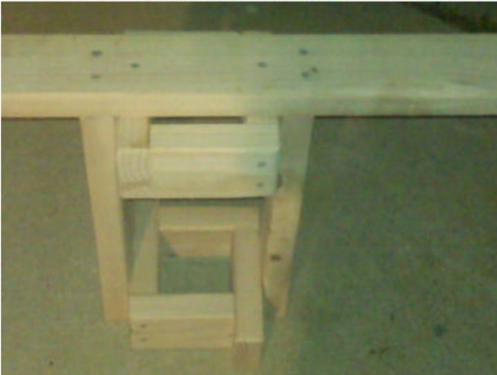
Attach the assembled piece to the center of one of the 6 foot pieces orienting the box with the protruding 2" X 4" opposite the 6 foot piece. (If you opted for the 45° bevels on one of them, you would use that piece here with the box assembly on the shorter side.)
