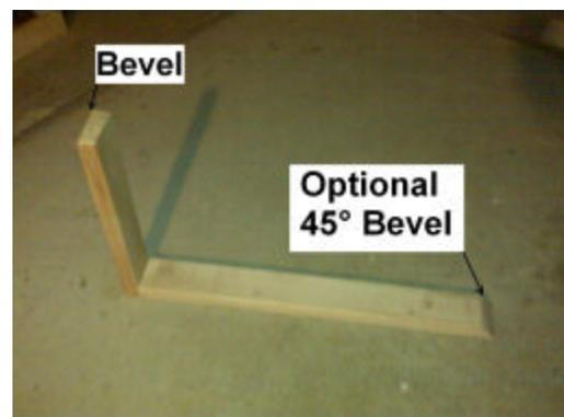
Attach the square end of the 18-3/8 inch piece perpendicular to the square end of the 31-1/16 inch piece with the slight bevel made in the previous step facing away from the 31-1/16 inch piece as shown. (If you opted for the 45° bevels on these pieces, the 45° angle will face up). Repeat this process for the other 18-3/8 inch piece and the other 31-1/16 inch piece.
