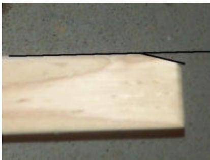
Using a belt sander or possibly a wood file if available, create a slight bevel on the wide side of one end of each of the 18-3/8 inch pieces as shown. This will make fitting the two base assemblies together a little easier.
