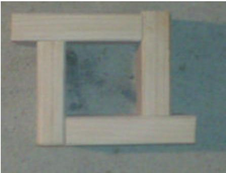
Attach the two remaining 5-1/4 inch pieces and the two 6-3/4 inch pieces in a similar fashion allowing the longer pieces to extend beyond the shorter ones (the shorter ones will butt-up to the longer ones 1-1/2 inch from the end.)
