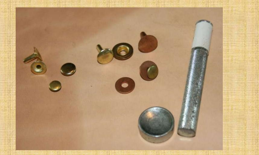
Chicago screws come in a variety of sizes, materials, and lengths. There are even extenders that can be added to existing **Chicago screws to let them** go through more layers of leather. Also Chicago screws are reusable and can be fastened and unfastened.
