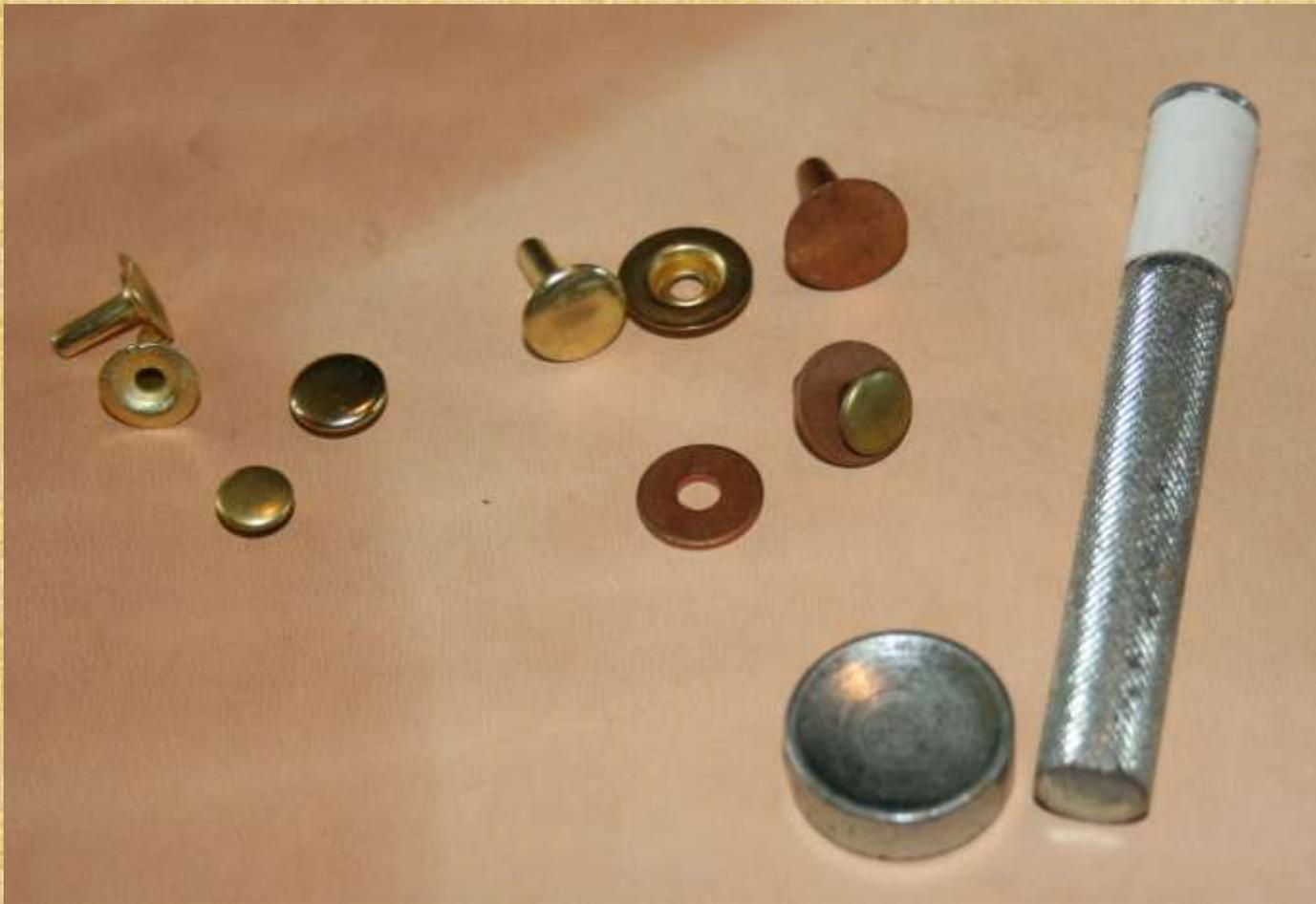
Chicago screws come in a variety of sizes, materials, and lengths. There are even extenders that can be added to existing Chicago screws to let them go through more layers of leather. Also Chicago screws are reusable and can be fastened and unfastened.
