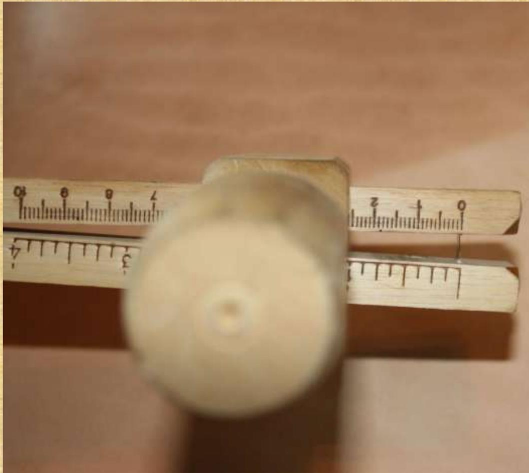
**Keep the strap cutter flush to the edge and draw along to leather.**
