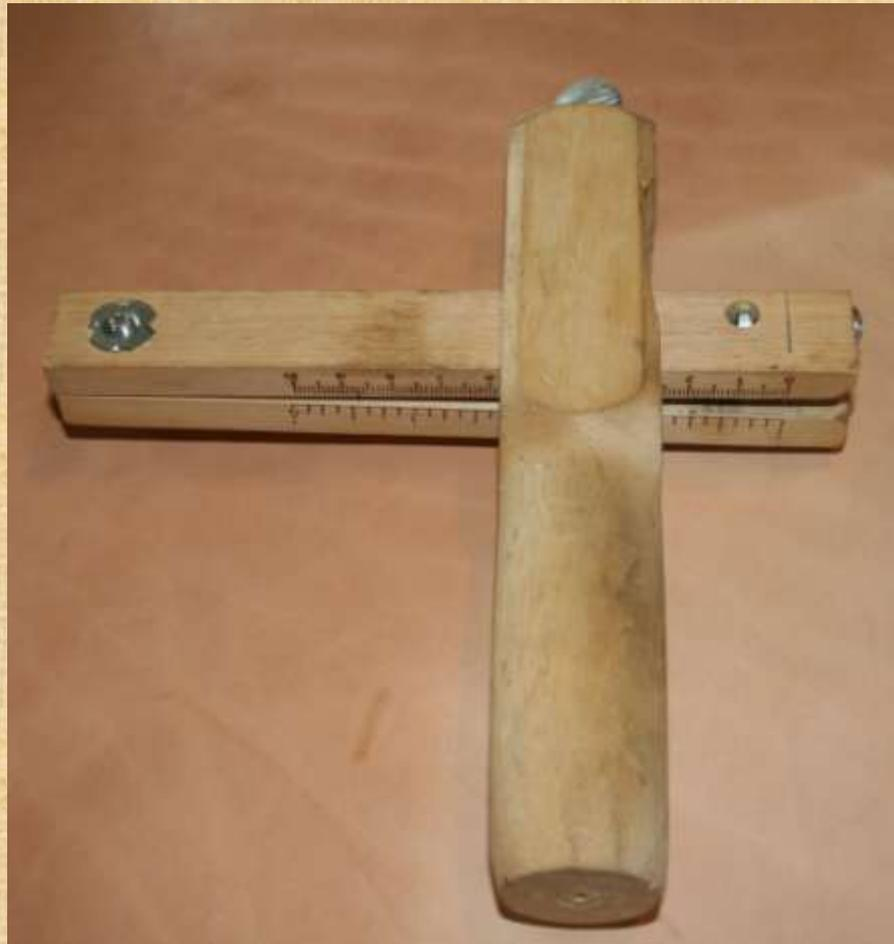
**Strap cutters can be adjusted by measurement.**
